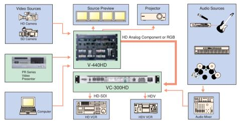
Figure 3. Production of live performance and studio video shot using various sources can be carried out using video mixing systems such as the Edirol V-440HD multi-format video mixer. If a VC-300HD is included in the system, the video line and audio can be combined during acquisition. Audio delay control, built into the VC-300HD, enables audio to be synchronized with the video.
